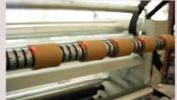
Laser indicators for quick positioning of cores.
