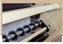
Knives are mounted on a driven shaft on a tangential slit configuration. Individual knife holders are available as an option.
