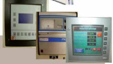
The Automatic tension and individual controlled rewinder rollers are all controlled by a single PLC. All controls are by way of a touch screen.
